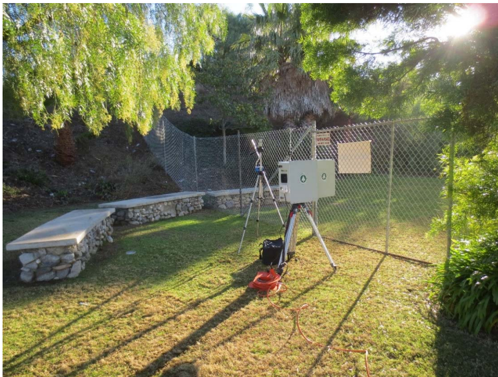
Photo 6: Pre-excitation: Setting up air monitoring stations (DTSC left, ENVIRON right) in front of temporary fencing by Building I.
