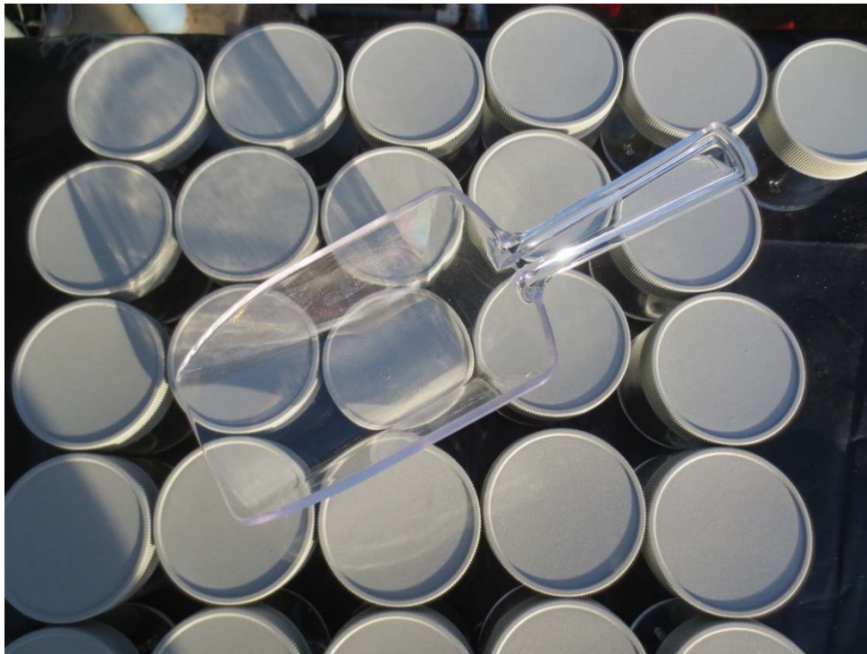
Photo 16: Sample jars and disposable sampler for post-excavation incremental soil sampling.
